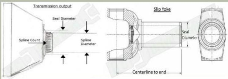
**Note:** GM TH400 with threaded hole in output shaft is 'Fixed Yoke' transmission and requires a .550" counterbored slip yoke, only available in Sonnax 1350 Chromoly Slip Yoke.
