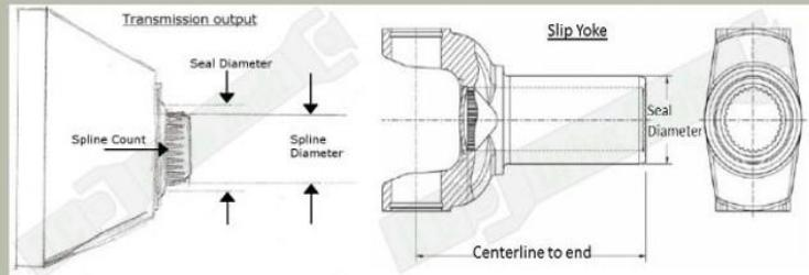
**Note:** GM TH400 with threaded hole in output shaft is 'Fixed Yoke' transmission and requires a .550" counterbored slip yoke, only available in Sonnax 1350 Chromoly Slip Yoke.
