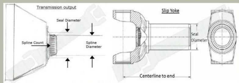
Note: GM TH400 with threaded hole in output shaft is 'Fixed Yoke' transmission and requires a .550" counterbored slip yoke, only available in Sonnax 1350 Mega Series.
